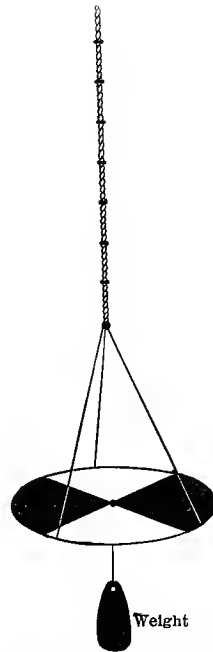
FIG. 48.—Disk for Comparing the Transparencies of the Water in Different Lakes.
