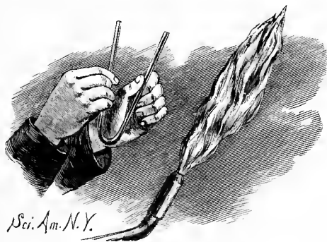
Bending a Glass Tube.
