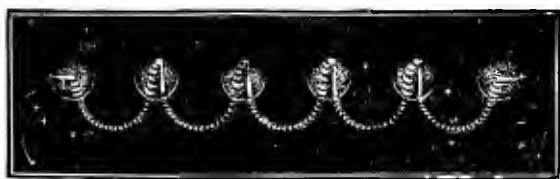
Geissler's Tubes showing Stratifications.
