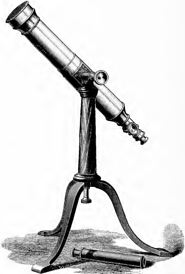
Compact Telescope— 2\frac{1}{2} inch Aperture, 24 inch Focus.
