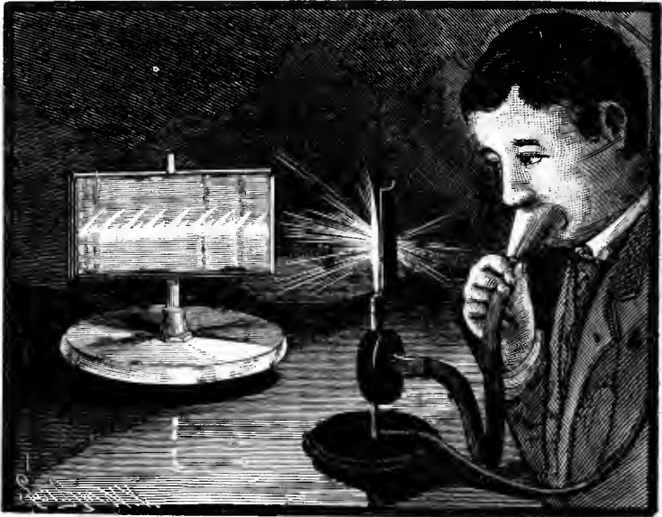
Top with Revolving Mirrors—Koenig's Manometric Flames.
