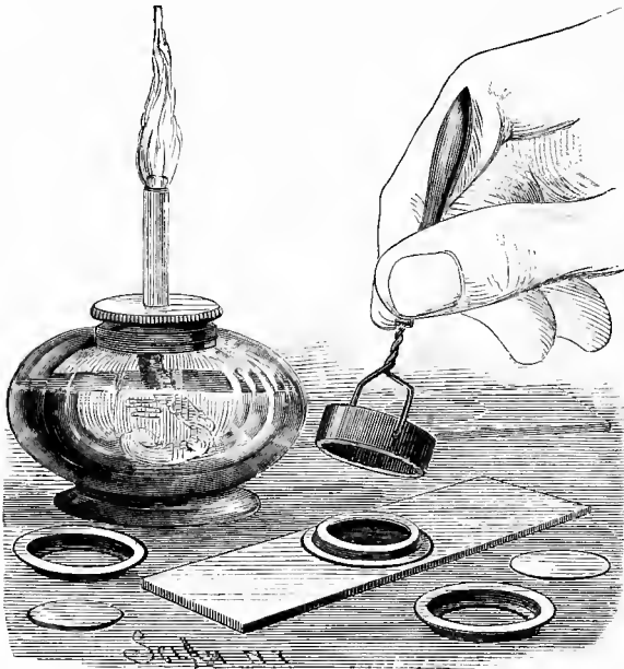
Quick Method of mounting Microscopic Objects.
