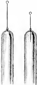
Sealing in a Wire.
