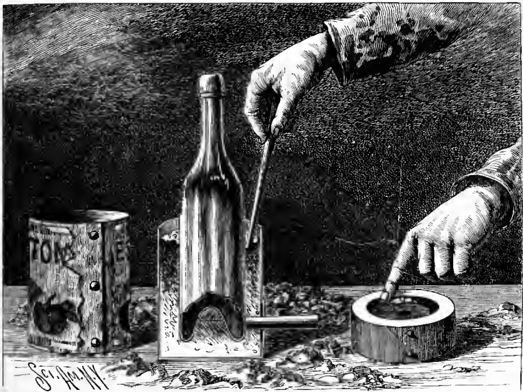
Making a Blowpipe Furnace.
