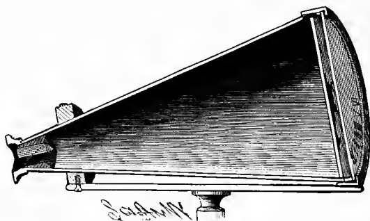
Longitudinal Section of Polar Clock.
