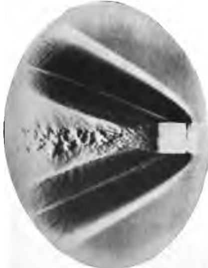
FIG. 148. —A near pointed brass projectile, showing head and tail waves travelling at the rate of 420 metres per second ( \times 2 diameters).
