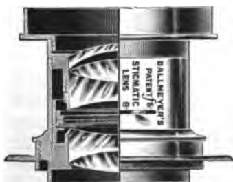
FIG. 91.—Dallmeyer's Stigmatic Lens. Entire lens as used for rapid or wide-angle work.
