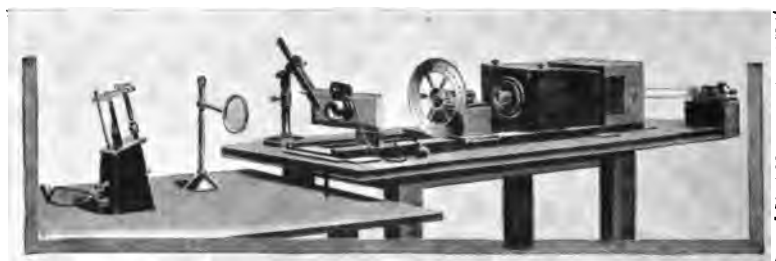
FIG. 152.—Sir William Abney's apparatus for determining the speed of a shutter.
