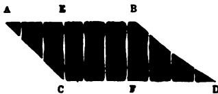
FIG. 153.—Time and Efficiency Record of the Opening of a Shutter, taken by Sir W. Abney's apparatus (Fig. 152).
