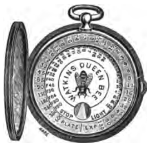
FIG. 160.—Watkins' Speed Measurer. 1
