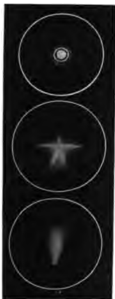
FIG. 99.—Appearance of coma and astigmatism together.
