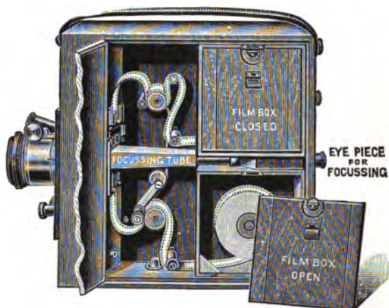
FIG. 28.—Interior Mechanism of Urban's Model D and DX Bioscope.
