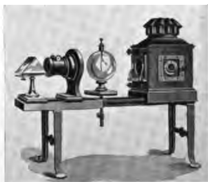
FIG. 181.—Hughes' Scientific Demonstrating Lantern for Institutes and Colleges, arranged with erecting prism.
