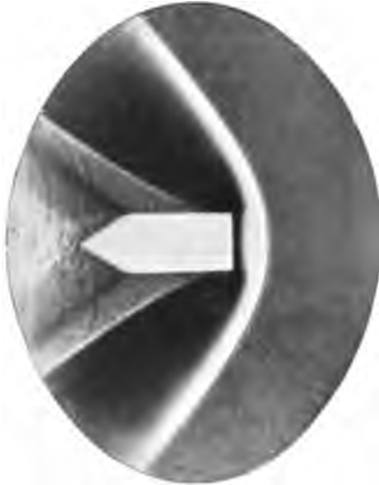
FIG. 147. —A blunt-nosed aluminium projectile travelling at the rate of 974 metres per second ( \times 2 diameters).
