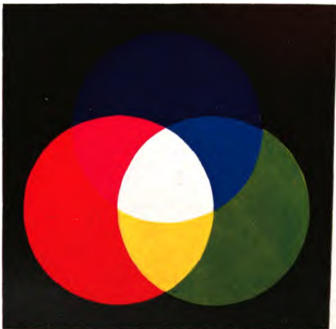
Primary colours. Diagram, showing the effect of superposition of "Additive" Lights , as explained on p. 222.
