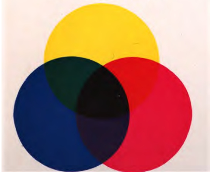
Primary colours. Diagram, showing the effect of superposition of "Subtractive" Colours , as explained on p. 222.
