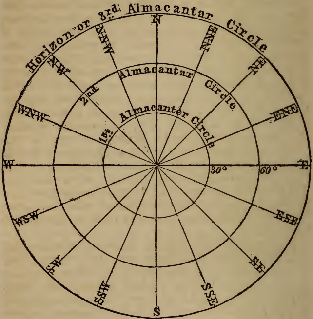
Fig. 9.—Points of the Compass. Terrestrial, Vertical Circles, and Almacantars.
