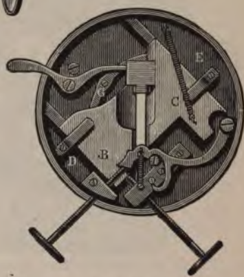
Section of No. 2100, showing slit mechanism.
