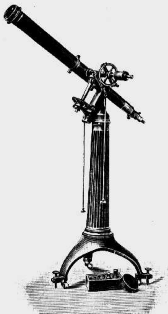
Fig. 25. Telescope on Iron Stand, with Divided Circles and Slow Motion.
