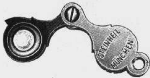
Fig. 15. Aplanatic Magnifier in Folding Mount
