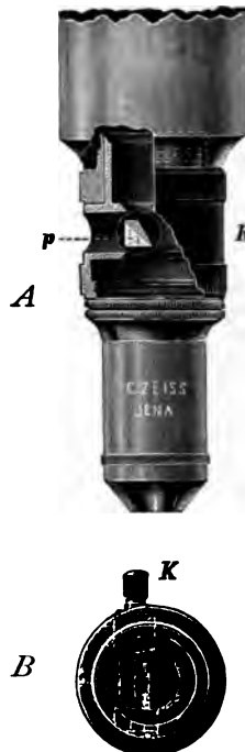
Fig. 31. Vertical Illuminator. A. View of same partly sectional showing the lower tube and the objective; B. Plan-view. ( \frac{2}{3} Full Size.)
