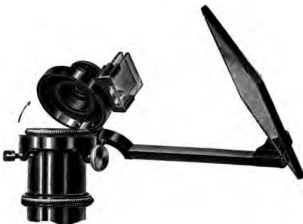
Fig. 44. Abbe's Drawing Camera No. 44. ( \frac{1}{2} Full Size.)
