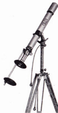
Fig. 9. Asegur. 2492 On extension rod with sun projection screen.
