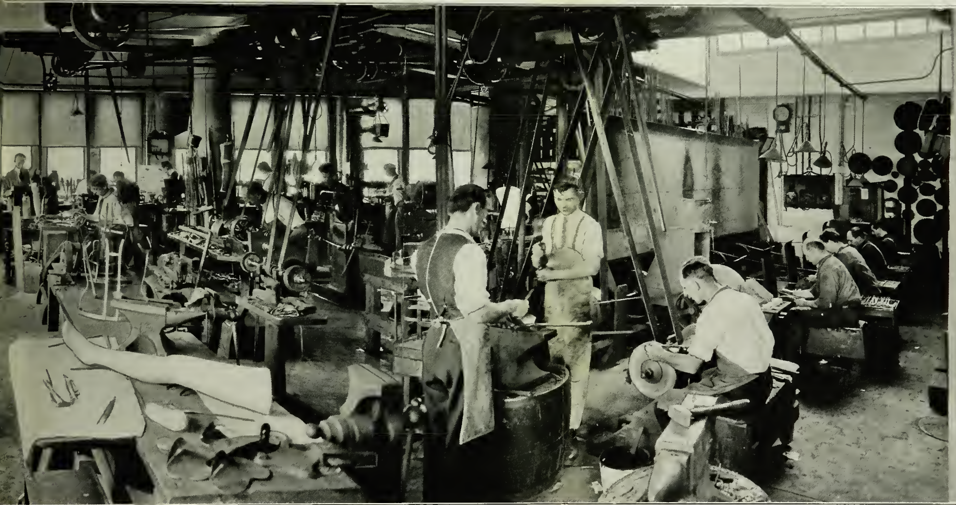
of Sixth Floor, for the making of Surgical Instruments, Orthopedic Appliances, Electrical Apparatus, etc. Here all Grinding, Polishing and Nickel-plating are done. All machinery is driven by electric motors.
