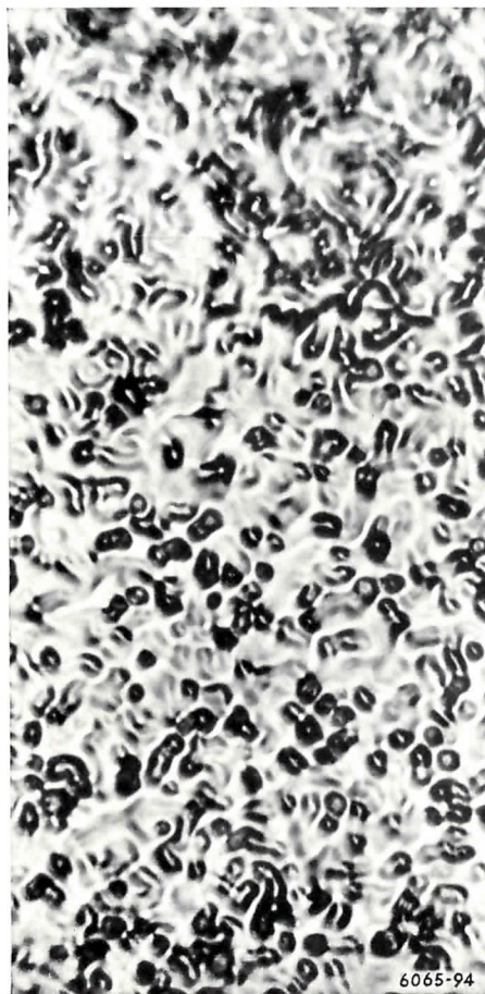
Fig. 2 After heating (1 hr.) to 1380 °C a closed surface has formed.
