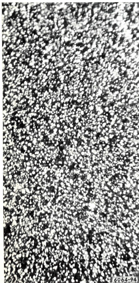
Fig. 1 Surface of a sintered tablet of carbonyl iron powder tempered in hydrogen. Initial temperature 20 °C (68 °F).
