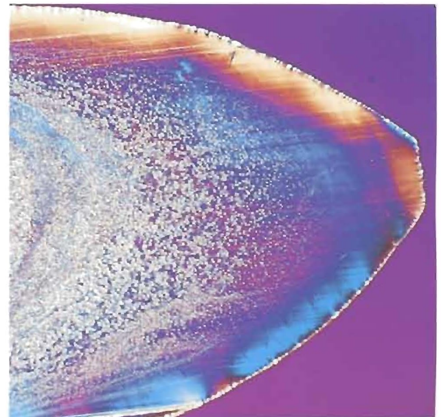
Plastic gear wheel, microtome section Photo: Dr. W. Patzelt, Wetzlar.
