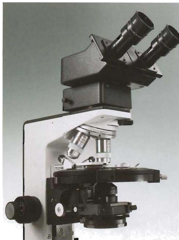
Fig. 7 LABORLUX 12 POL S, Pol tube S 20, intermediate tube 90B, strainfree objectives, removable stage, PLK Pol condenser.
