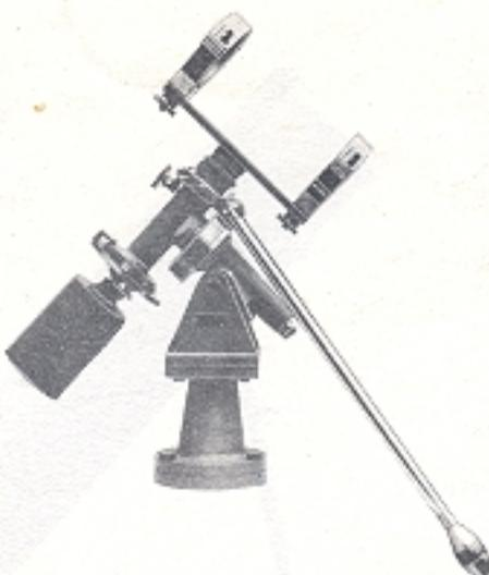
These mountings are fitted with one slow motion drive and driving handle, release clamp for fast movement and adjustment for latitudes. Also provided are bands for holding telescope and counter balance weights. Iron columns or tripod stands can be quoted to suit customers requirements. Degree, Hour Circles and Verniers provided.
