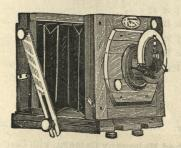
Consist of a Superior French Polished Mahogany Bellows-body Camera, having screw adjustment for Focussing, Swing Back, Vertical and Horizontal Sliding Front, One Hinged Double Back, Achromatic View Lens with Instantaneous Shutter, and Set of Rotating Stops, and Mahogany Tripod Portable Stand, or a Cycle Clip.
