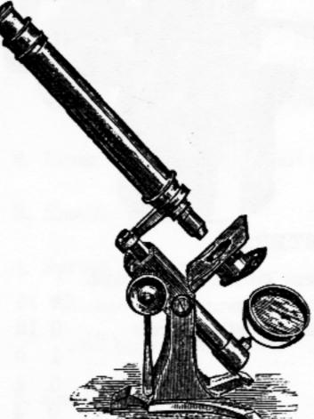
This stage has 1-inch motions in rectangular directions by levers, and having no milled heads, it can be advantageously used with the largest Zoophyte trough or stage plate.
