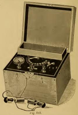
In Walnut-wood Case, with Switch, Cell Selector, Galvanometer, Current Reverser, Improved Handles and Cords (Fig. 818).
