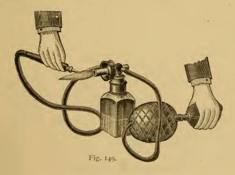
This new apparatus claims the following advantages:—The Spirit Lamp is entirely dispensed with. It can be put away inside the case complete in working order, without the possibility of the Benzoline being upset.
