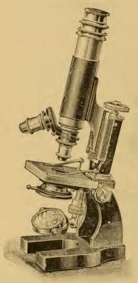
Very firm and compact horse-shoe stand, with inclining joint, English pattern (as drawing), of highly-finished brass, best fine adjustment, revolving diaphragm to stage, swinging substage with screw adjustment, one eye-piece, iin. object-glass magnifying to 80 dias, and 6 in. object-glass (0.74 N.A.) magnifying to 400 dias in mahogany case.
