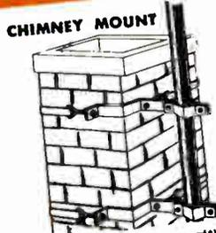
Can be erected in minutes, without special tools or drilling. Adjustable, two-section design permits unlimited spacing between brackets for maximum support of masts 1/2" to 1 1/4" O.D. Complete with two 12-ft. lengths of 1/4" galvanized steel bands and hardware.
