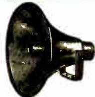
**REFLEX LOUDSPEAKER TRUMPETS.** For use with driver units below. Fully weatherproof. Heavy-gauge metal. Model GH with 6 1/2" air column and a low-frequency cutoff at 85 cps is ideal for music, models LH and PH have higher cutoff for general use. Model SMH is for voice only. With "U" mounting bracket, less driver unit.
