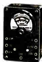
Pocket-sized. Handy for use in communications service, schools, radio service shops—wherever a small but durable unit is required. The 2" flush mounting meter is a permanent magnet, iron vane, solenoid type. Uses two standard flashlight cells. Range: DC volts, 0-3-15-30-300. DC ma., 0-25; Ohms, 0-10,000. Housed in molded bakelite case, with bakelite panel. Ranges selected by phone-tip jacks. Size, 1 1/4 x 2 1/4 x 3 3/4". With batteries, less leads. Shpg. wt., 1 1/4 lbs. **NET... 6.86**
