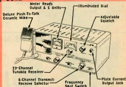
Volume, Squelch, Tuning, Spot Switch, Channel Selector, Meter Switch, Tune-Fixed Selector, Earphone jack. Built-in 3" Speaker. For 117V AC. 15-tube function. Tubes: 6DS4 (Nuvistor), (2) 6EAB/6U8A, 6AU6, 6T8, 6AQ5A, 6AW8A, IN34A silicon diode doubler. Includes set of crystals for Channel 9, Push-to-Talk highly dependable ceramic mike and coiled cord with plug. 11 1/2 x 5 x 6 3/8". Shpg. wt., 14 lbs.
