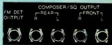
FM Detector and "SQ"/COMPOSER Decoder Outputs (Rear).
