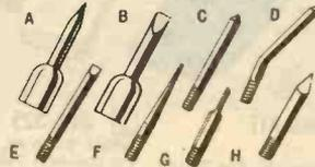
Thread-in and thread-on soldering tips. Made of super tough copper alloy. The PL series is iron clad and silver plated. Others are unplated. The 100 series Mini-Tips, 3/4x1/8" O.D., are used with 1237 and 4037 units only. The 300 series tiplets, 1Lx1/4" O.D., are used with heating units 535, 1235, 4035 and with the Princess soldering irons. The 800 series Tiplets, 3/4" O.D. for high heat transfer, are used with the 4045 unit. 833 and 834 1 1/4" L, 823 and 824 are 1" L. Avg. Shpg. wt., 3 oz.
