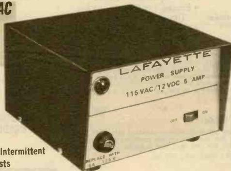
Double the use of a car stereo tape player by using it in your home or office. Converts 115 volts AC to 12 volts DC. Handles a maximum load of 5 amps. Features on/off switch, heavy duty color coded binding posts, neon indicator light, and accessible fuse in front. Black metal cabinet. For 117 VAC, 60 Hz. Size: 4<sup>9</sup>/<sub>8</sub>"W x 6<sup>1</sup>/<sub>2</sub>"D x 3"H. Shpg. wt., 6 lbs. Net 15.95
