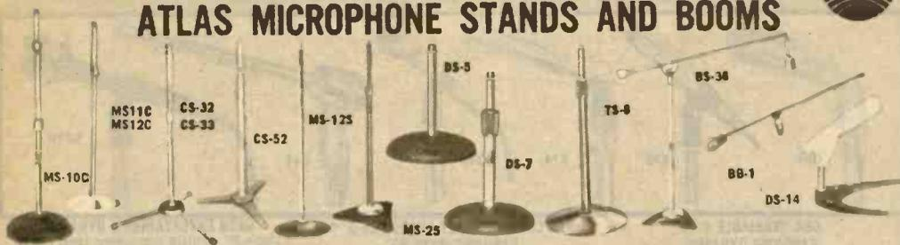
**Model MS-10C Full Grip Mike Stand.** Economical mike stand featuring "Full-Grip" clutch mechanism for fast quiet adjustments without slipping and wear. Functionally designed base assures maximum stability and includes self-leveling, shock-absorbing pads plus 3 "anti-tip" points. Full chrome plated tube assembly. Terminates in a  $\frac{3}{8}$ "-27 thread. Base dia. 10", finished in gray shrivel. Height adj., 35 to 63". Shpg. wt., 10 $\frac{3}{4}$  lbs.
