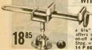
For small sub-assemblies and intricate electronic work including printed circuits. Rubber protected jaws are 2 1/8" W with a 6 1/8" opening. PowRarm positioner offers superior positive lock and fast on-off action with horizontal handle. Shpg. wt., 2 3/4 lbs.
