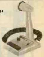
The "Plus-3" ceramic microphone has a new transistorized pre-amp with volume control plus a new compression amplifier circuit which allows user to talk close or far from the mike without varying the output signal. This prevents mike sput and sputter. Response: 300-3000Hz. 3 conductor (1 shielded) coiled cord. Touch-to-talk front bar switching with slide lock when desired. Wiring instructions for over 100 popular transceivers. Shpg. wt., 4 lbs.
