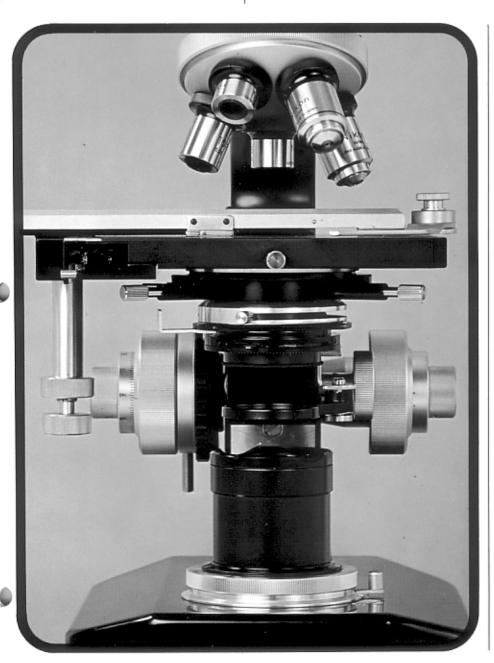
The range of condenser focusing is 28mm with rack and pinion motion. The condenser holder accepts various condensers, bright-field or dark-field, including the long focal-length condenser specifically developed for tissue culture studies. Centering is accomplished by means of radial screws in the substage to accurately align the optical axis of the objective to the built-in illumination system.
