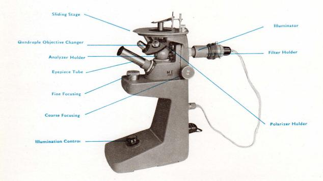
Basically the ME is an inverted microscope of compact and of very original design. The self-contained illuminator is good and a transformer for varying the intensity of the illumination is built into the base of the stand.
