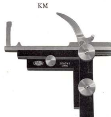
Ungraduated mechanical stage Model KM Range of operation: 75x25mm
