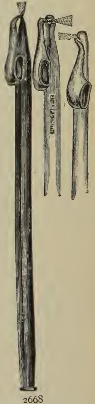
Figure 2664-a. Rumbold's Spray Controller. a , set-screw, to control the pressure on the rubber tube connected with the compressed air reservoir. The illustration shows the manner of holding the instrument. The Spray Controller is thus made the handle of the Spray Producer.
