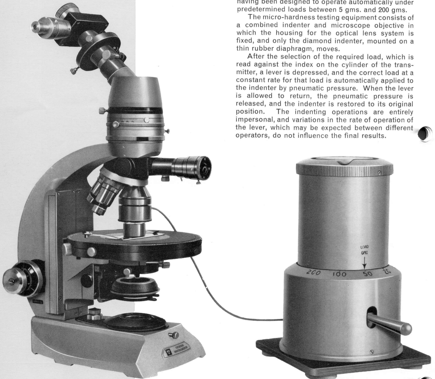
M74 polarizing microscope with micro-hardness testing equipment.
