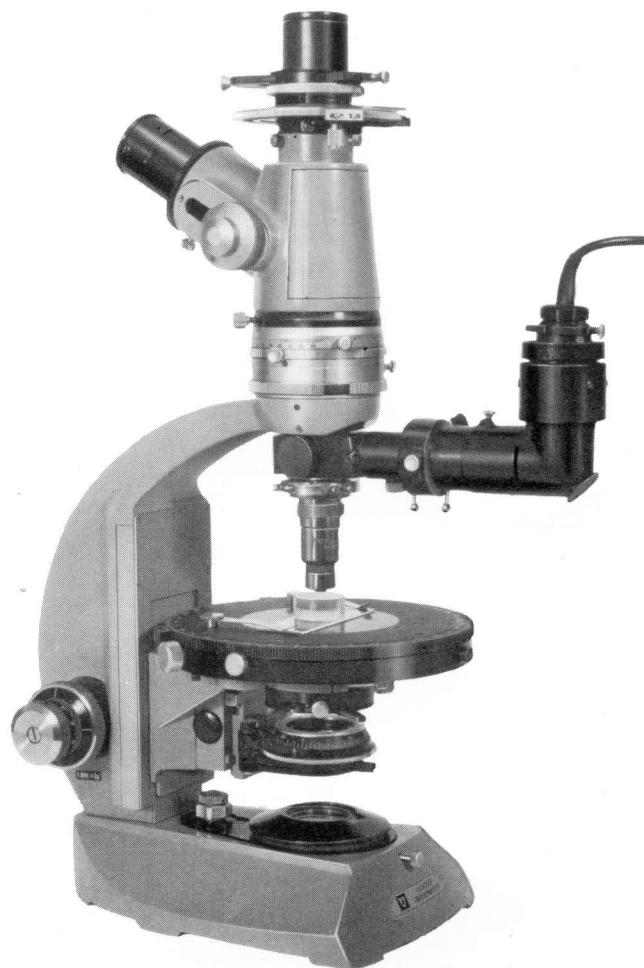
M74 polarizing microscope with M730150 built-in incident illuminator and Dick-Wright ocular.
