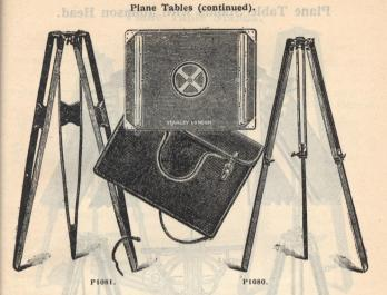
P1080 Plane Table, Government Portable Pattern, with sliding leg stand, Sequoia board, 18 × 18 inches, with aluminium battens fitted by an improved method to allow the board to expand and contract with atmospheric changes, aluminium corners and racer ring. Complete in waterproof case with carrying strap, sliding stand in oiled teak, as illustrated .....
