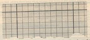
For plotting longitudinal sections of railways, roads, etc., without the use of scales. The ruling is to the scale of 20 feet to 1 inch horizontal, and 4 feet to 1 inch vertical.
