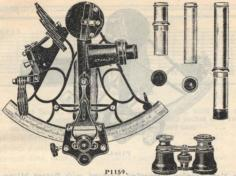
The Stanley Mark 3E "Bell" Sextant, 7-inch radius, P1159 divided on silver to 150° and reading by vernier to 10 seconds. Accessories : Star Telescope, power × 3, Inverting Actro-matic Telescope, powers × 6 and × 10, sighting tube, star binoculars and two eye-shades, with endless tangent motion, and packed in hardwood case polished inside and out, with lever lock. Complete with N.P.L. CLASS "A" CERTIFICATE 22
