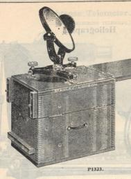
P1323 Heliotrope, Government pattern, consisting of 6-inch mirror with horizontal and vertical rack and pinion adjustment, sight hole and levelling screws, in strong wooden case, which 13 0 0 is used as a stand for the instrument 10.14
