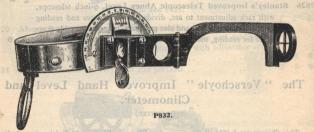
This instrument does the work of an Abney Level, Clinometer, and Prismatic Compass. It was designed by Mr. W. D. Verschoyle, a mining engineer of great experience, and has since become known as a very complete Pocket Surveying Instrument. By its use only one observation is necessary to obtain the vertical angle and magnetic bearing of any object.
