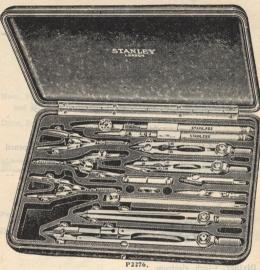
P2276 Perma Pocket Case, containing the following first quality instruments :-Compasses, 6-inch, double jointed, with shouldered needle points, pen and pencil points, and lengthening bar (P2251).
