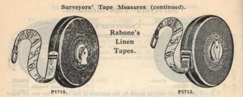
N.B.—Linen Tapes will all vary in length by the moisture of the air. They are all tested to standard before delivery. Unless otherwise ordered, Feet Tapes are marked on the back in links, and Metre Tapes have English feet and inches on reverse side.
