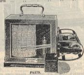
P6175 Hygrograph, recording wet and dry temperatures, Meteorological Office Pattern, with exposed laminae, which ensure perfect circulation of air, metal hinged case, enamelled iron base, seven-day clock, 6-inch setting thermometer for purposes of comparison, 11×7½×5 inches, weight 9½ lbs.
