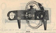
A point that distinguishes this instrument from all other well-known types at present on the market is that all delicate parts are enclosed, and only the very roughest usage will put it out of adjustment.
