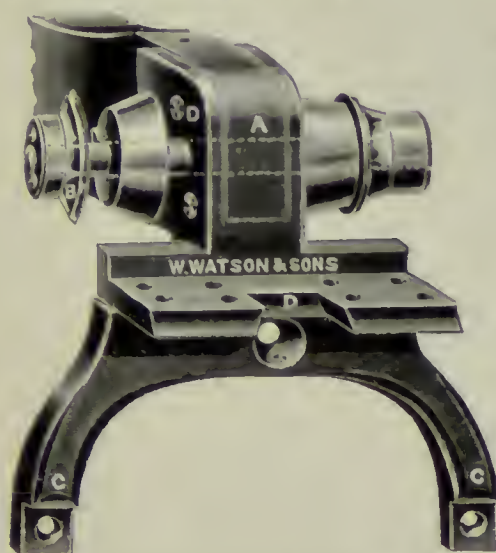
View of the method of fitting the Stage and Limb in the Van Heurck Microscope.
