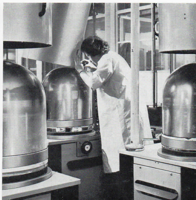
dielectric coating of lenses and mirrors . . .
