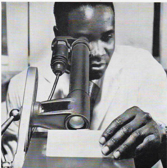
checking the angle of a prism...
