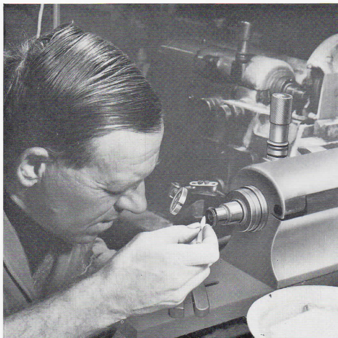
Truing a lens preparatory to edging ...
