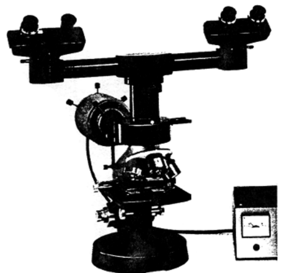
Wild M12 microscope with 12V/100W incident light attachment, discussion tube 256 547 and observation tubes. The left is the inclined binocular tube G, the right is the inclined binocular tube G 256 519 with both eyetubes adjustable
