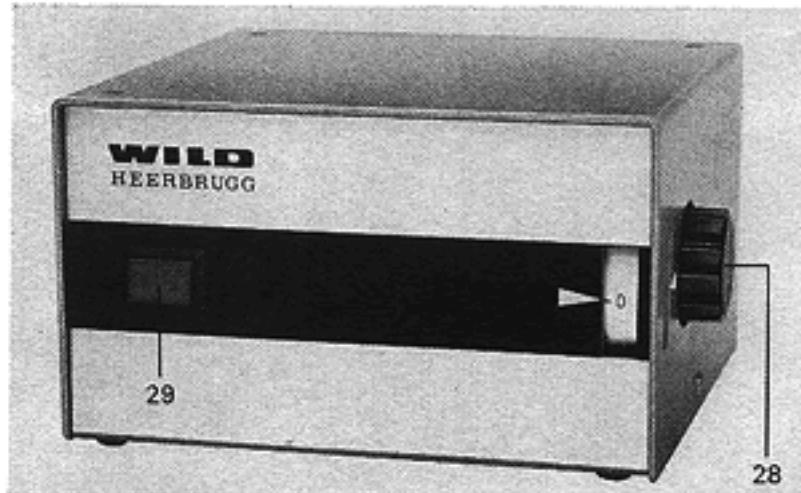
Set the regulating knob (28) of the transformer to '0' and connect the mains (line) lamp to the electricity supply. Switch on the transformer by depressing the luminous key (29). Turn the regulating knob (28) until the required brightness is obtained.
