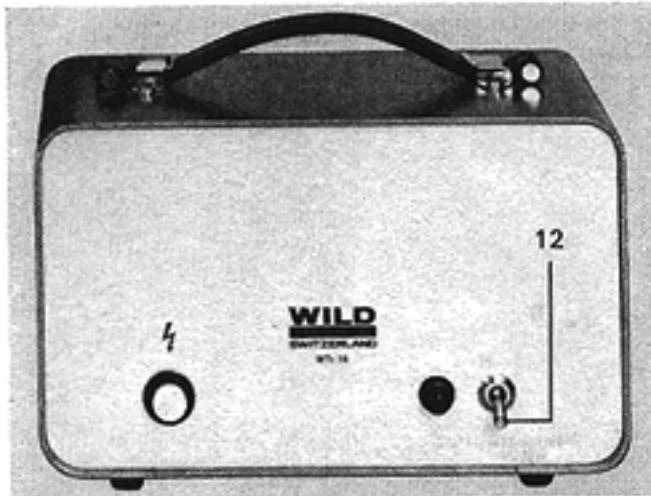
Flick the mains (line) switch (12) upwards to turn it on, and depress the ignition key ( $\leftarrow$ ) for 5 to 10 seconds. While the ignition key is depressed the pilot lamp does not shine. Allow the burner to warm up for a few minutes. It may happen that a new burner will ignite without the ignition key having been depressed. The key should be depressed nevertheless, so that the burner warms up as soon as possible.
