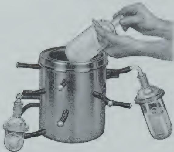
These VirTis Freeze-Dryers are self-contained, compact units, designed for the utmost in efficiency. The center well, filled with dry ice and solvent, acts both as a condenser and as cold bath for initial "shell-freezing". When frozen, the flask of material can be quickly hooked up to one of the vacuum ports.
