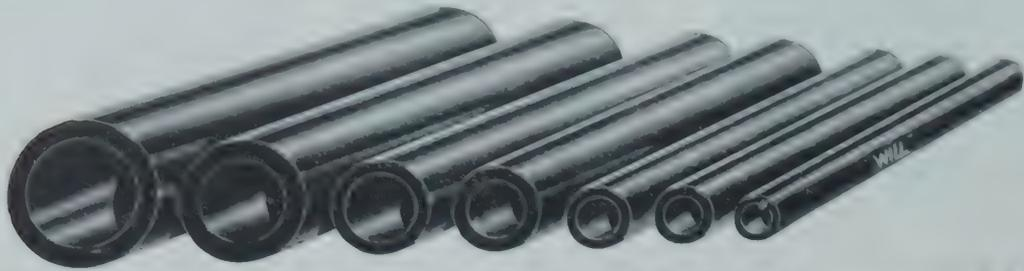
**23451 RUBBER TUBING—Pure Gum, Medium Wall, Black.** A seamless, hand-made, cloth impression tubing made from the finest Para rubber, steam-cured, and especially durable under laboratory conditions. It meets Federal specifications for Grade A pure gum tubing, has a very low sulphur content, a specific gravity of 0.97, high tensile strength and excellent aging characteristics.
