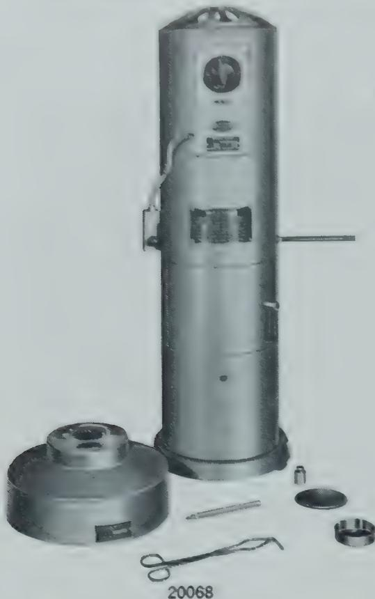
**20068 SOLIDS DETERMINATOR—Dietert.** For the determination of solids in milk products. This determinator is highly accurate, fast and simple to operate. The equipment is compact and requires little space. The basic units include:
