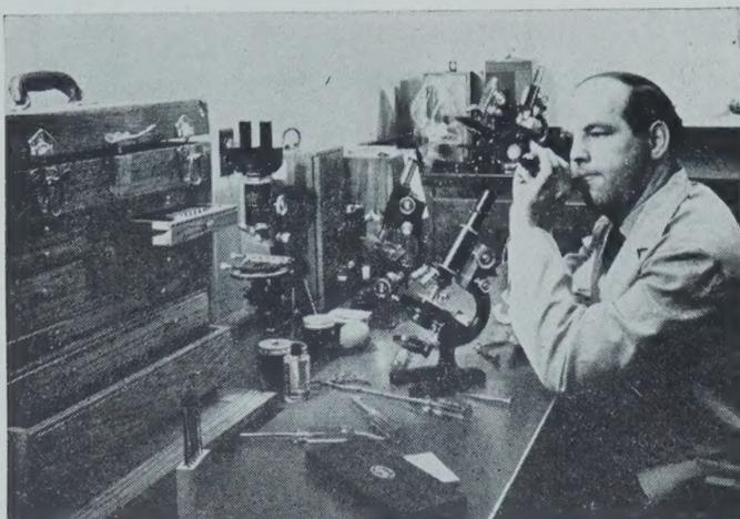
*Microscope repairs at our Rochester Service Center.*
