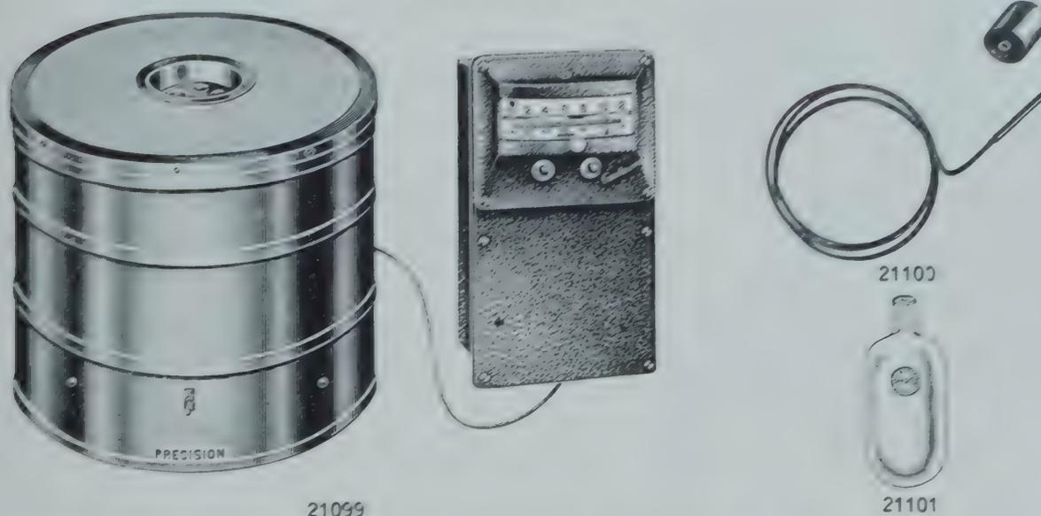
**21099 CARBON RESIDUE APPARATUS—Ramsbottom, with Automatic Pyrometer Control.**
