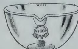
**11091 DISHES—Evaporating, "PYREX" Brand Glass (Corning No. 3180).** Made with flattened bottom for stability and for increased contact surface on a hot plate. They have a well-formed pour-out, frosted circle for pencil identifications, and they may be used at elevated temperatures over a free flame.
