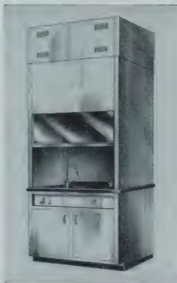
**CLOSED TYPE FUME HOOD** with enclosure above chamber for concealing blower and ducts. 47 in. wide, 30 in. deep and 10 feet high. Exterior of heavy gauge reinforced steel. Interior of the Fume Hood chamber of treated transite panels, accurately cut, tightly fitted and cemented. Supplied with duplex receptacle, gascock with remote control valve, gooseneck water fixture, lead bowl sink, fluorescent light.
