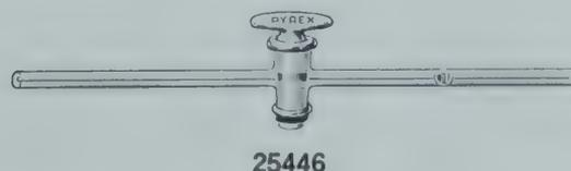
**25436 STOPCOCK—Glass, Capillary, Straight Bore.** The inlet and outlet tubes are capillary tubing having an outside diameter of approximately 7 mm. and 2 mm. bore. The solid glass plug is carefully ground-in, and has a bore of 1½ mm. and is equipped with rubber retaining washer..... 1.87
