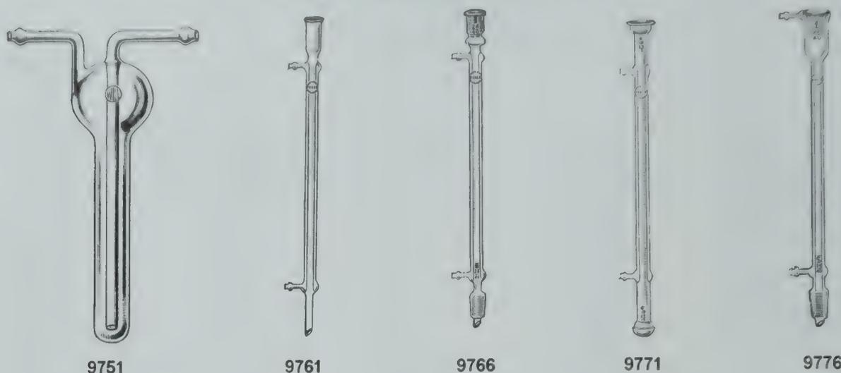
**9751 CONDENSER—Reflux, "Cold Finger."** Used in the necks of flasks for condensing and refluxing vapors. It may be employed without stopper, loosely fitting the flask neck, and has proved very convenient for a number of laboratory operations. The lower section for insertion in the flask neck is 20 mm. in diameter and 120 mm. long with a bulb diameter of about 45 mm.
