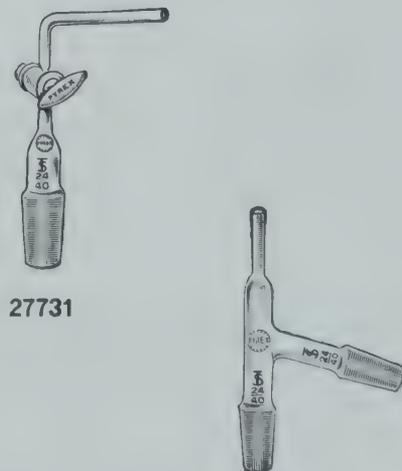
**27736 TUBES—Connecting, Two-Way, Standard Taper, "PYREX" Brand Glass, with Thermometer Opening (Corning No. 8960).** These tubes have inner Standard Taper joints of the same size on the lower end and side arm, with a plain top opening at the upper end for the insertion of a thermometer. The side tube is attached at an angle of 75°.
