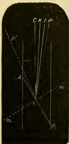
Path of the rays with different cementing media. COA limit of the field for Canada balsam, KOA for balsam of copaiba, IOA for linseed oil, POP' for poppy oil; mm. direction of the axis of the crystal.
