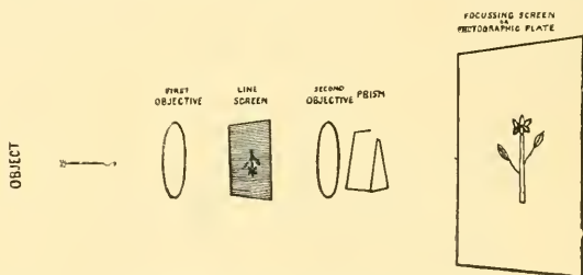
FIG. 82.—General optical arrangement shown diagrammatically.
